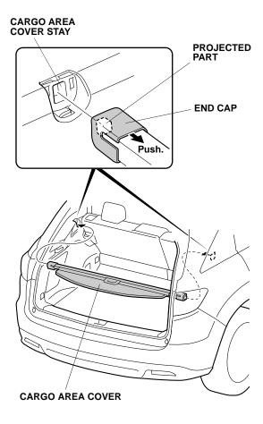
4. Pull out the cargo area cover and secure the two tabs into the channels in the rear side lining as shown.
